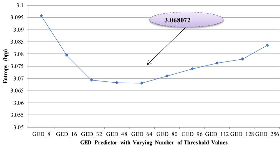
Figure 6. Average value of entropy from GED predictor with varying threshold values for R2 resolution.
