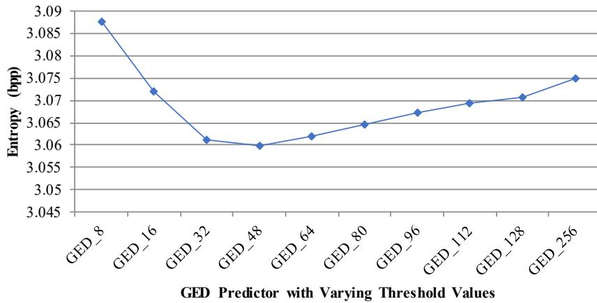
Figure 8. Average value of entropy from GED predictor with varying threshold values for overall dataset including different resolutions and different modalities.
