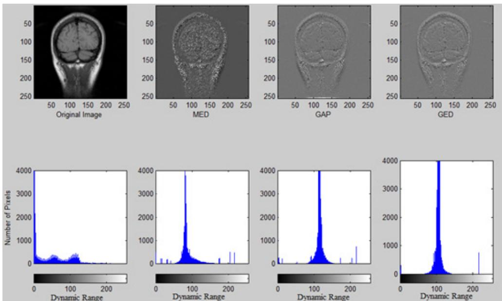
Figure 4. Original MRI-scan image of brain, residual image obtained from MED, GAP and GED predictors and their histograms
