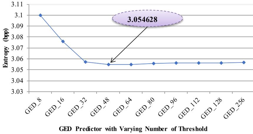
Figure 7. Average value of entropy from GED predictor with varying threshold values for image resolution in between 256×256 and 512×512
