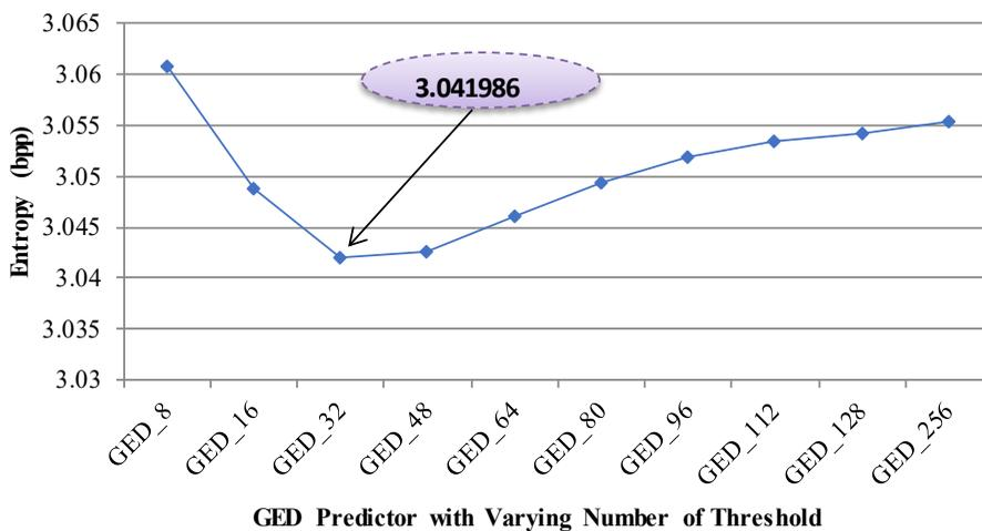
Figure 5. Average value of entropy from GED predictor with varying threshold values for R1 resolution.
