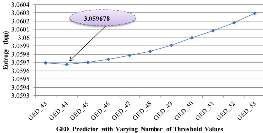
Figure 9. Average value of entropy from GED predictor with varying threshold before and after threshold point 48 for complete set of different modalities of medical images.
